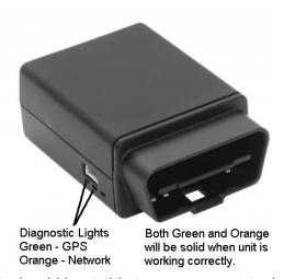
When the lights are solid, the unit should be visible in your account in the GPS Tracking system. When first installed, it may take several minutes for the unit to show in the system.
